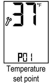
As long as the ambient temperature is lower than the temperature set point P01, the heaters will turn ON upon receiving a positive snow signal from the snow detector.
