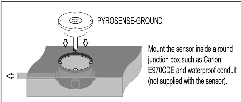
Mount the sensor inside a round junction box such as Carlon E970CDE and waterproof conduit (not supplied with the sensor).
