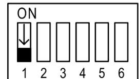
**Important: Changes made to technician parameters will not take effect as long as DIP switch S1 is in ON position.**
